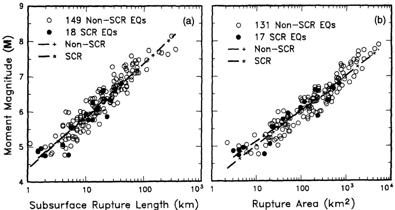
Figure 17. Regression lines for stable continental region (SCR) earthquakes and non-SCR continental earthquakes. (a) Regression of surface rupture length on magnitude ( $M$ ). (b) Regression of rupture area on magnitude ( $M$ ).
