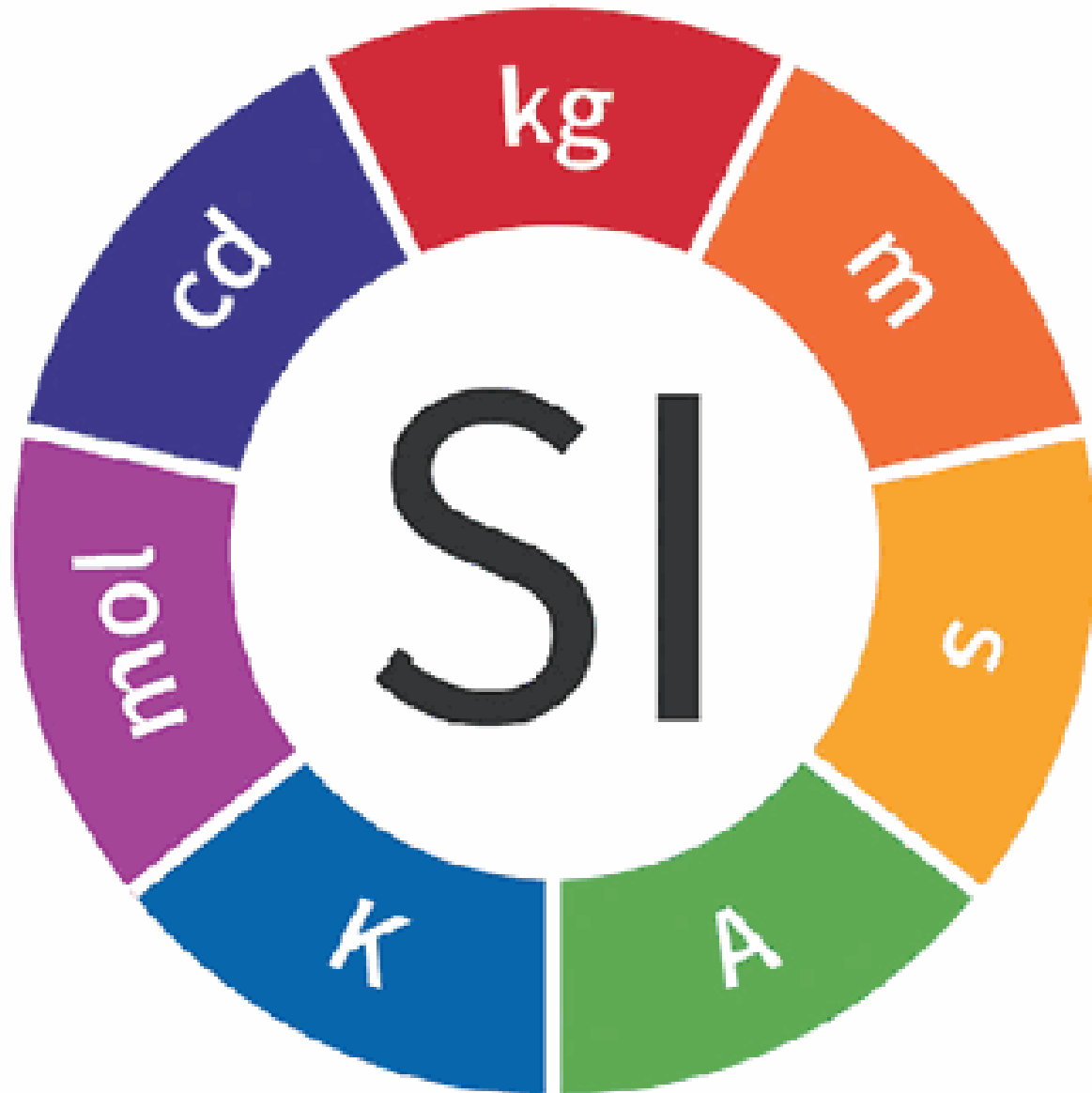
Figure B3.1 Logo for SI with base unit abbreviations for the kilogram, meter, second, ampere, kelvin, mole, and candela. ( candela is unit of luminous intensity )
